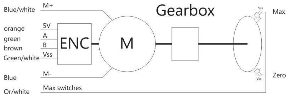
Connection of Huafang Slewing drive motor SE3C-62-R-24E005
